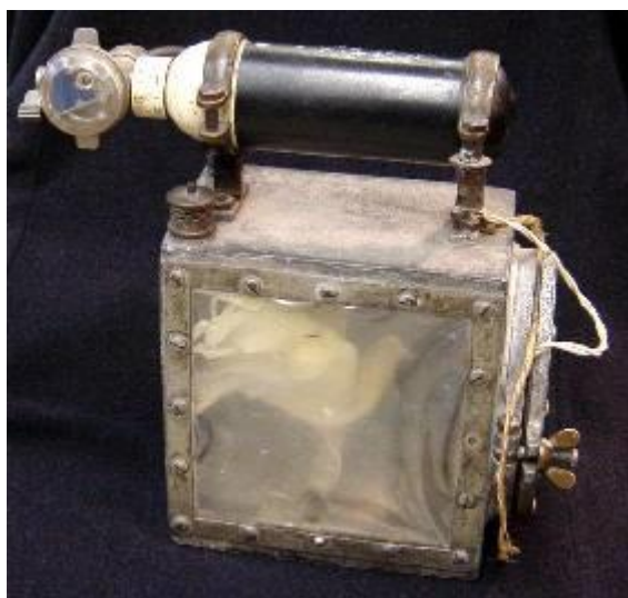
Canary cage with oxygen-cartridge made in England by Siebe-Gormann, found in Australia (used in the Broken Hill Mines)
