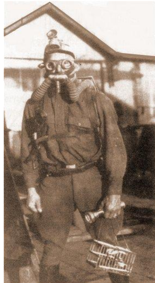
...preparing to enter the collapsed mine shaft of the Argonaut Mine; Courtesy National Archives Left: An early attempt at a combination illumination and gas testing device.
