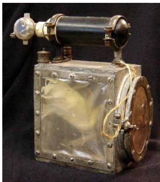
Canary cage with oxygen-cartridge made in England by Siebe-Gormann, found in Australia (used in the Broken Hill Mines)
