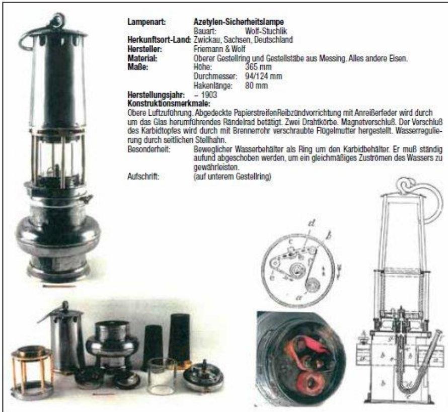
3 Azetylen-Sicherheitslampe, Bauart: Wolf-Stuchlik
