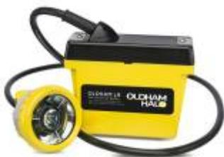
The heart of the D-series of mining lamps is the 3-Watt side-emitting power LED that is run at a genuine 3 watts. The light from this source is focussed by a unique reflector that gives a spot of 5000 lux at 1 metre and 10 Cd over 120 degrees, surpassing performance levels of all competitor LED powered lamps. [Products from Oldham today](#)
